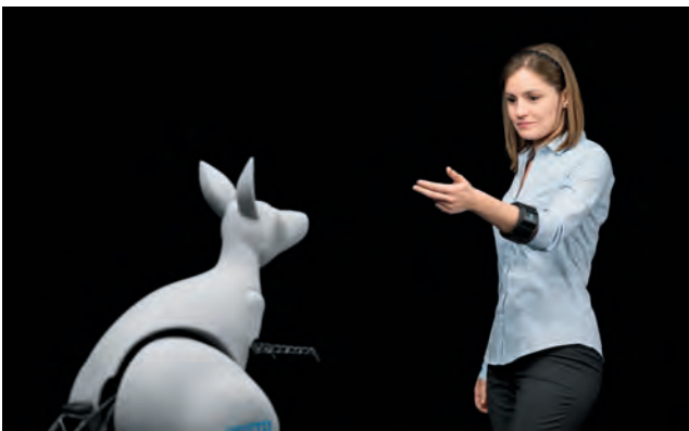
Simple operation: gesture control using armband
